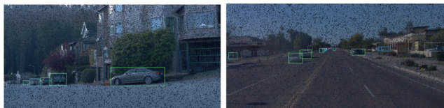
FIGURE 10. Image - Waymo - spatter test case. White: Ground truth boxes. Green-to-blue: more uncertain detections.
