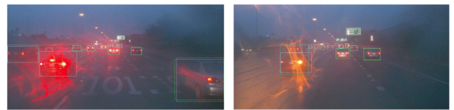
FIGURE 7. Image - Waymo - rain test case. White: Ground truth boxes. Green-to-blue: more uncertain detections.
