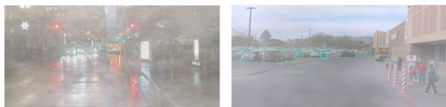
FIGURE 11. Image - Waymo - fog test case. White: Ground truth boxes. Green-to-blue: more uncertain detections.
