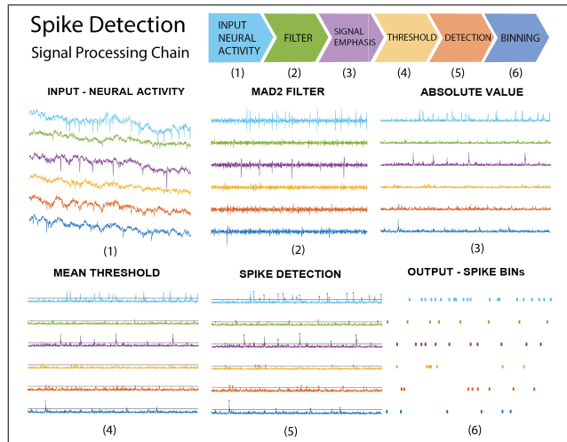
FIGURE 2. The input neural activity (1) is processed by five pipelined modules: the MAD filter removes the low-frequency components (2); the signal is rectified by the spike emphasis module (3); the mean of the rectified signal is used as a basis to compute the threshold (4) to detect the spikes (5); one-millisecond spike bins are forwarded in output (6).
