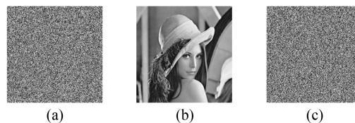
FIGURE 11. Key sensitivity experimental results (a) ciphertext image, (b) decrypted image with the correct key, (c) decrypted image with the incorrect key.
