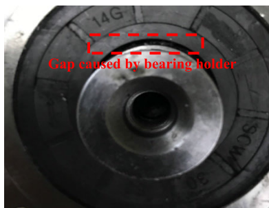
FIGURE 22. The fault caused by the bearing holder fracture.
