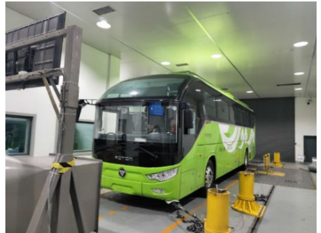
FIGURE 13. Rotary hub test of sample vehicle.
