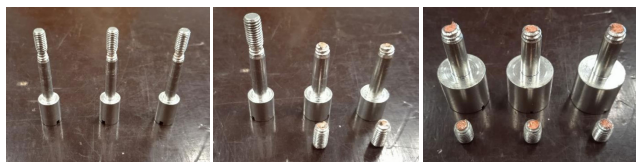
FIGURE 38. Samples of bolts after tensile test.
