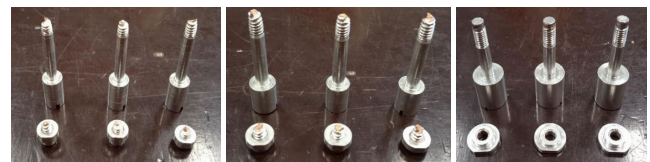
FIGURE 37. Screw connections after tensile test.
