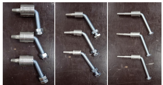
FIGURE 40. Samples of bolts after bending test.
