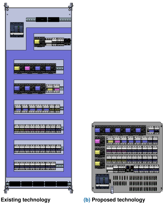
FIGURE 1. CAD model of mounting plates incorporating the same equipment.
