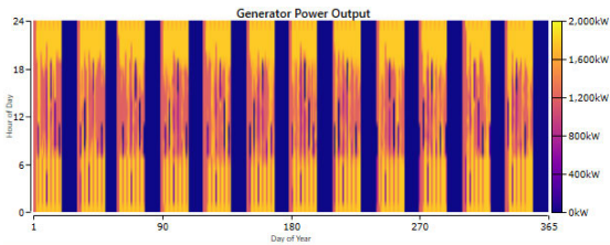
FIGURE 13. The diesel generator output at 900 kW PSCs.
