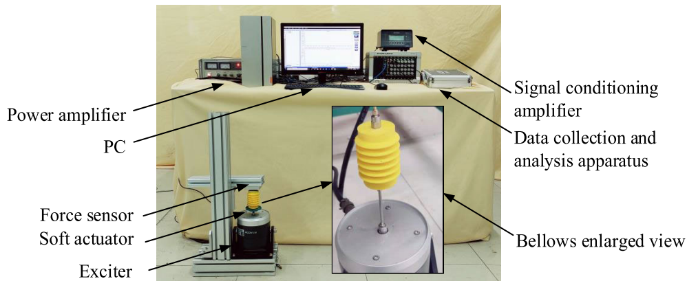
FIGURE 3. The dynamic experimental device of the dual-chamber flexible bellows isolator.
