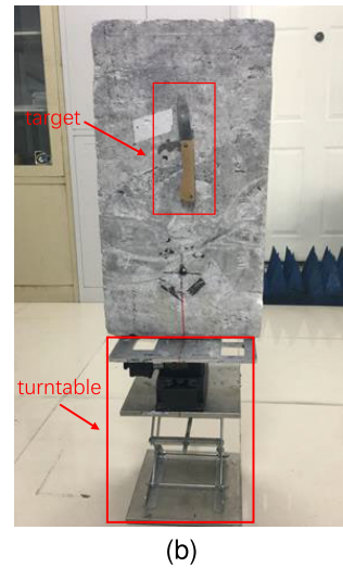
FIGURE 14. (a) Experimental scenario for generating the multi-plane MIMO array, and (b) photograph of a fruit knife fixed on the turntable.
