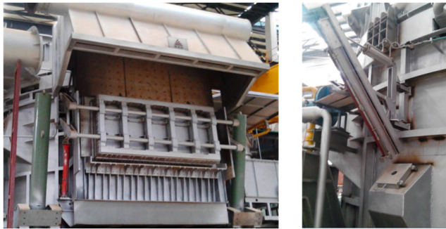
FIGURE 3. Pictures of furnace door and liquid aluminum temperature thermocouple.
