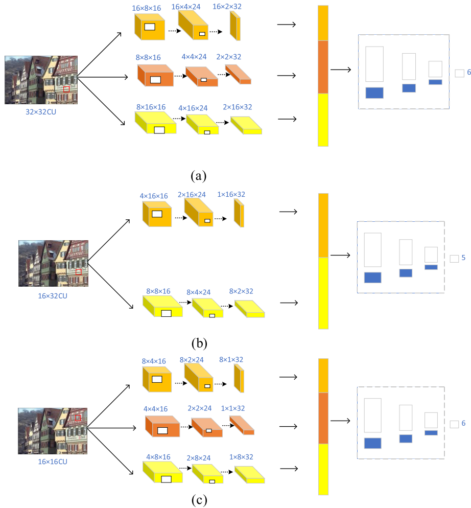
FIGURE 3. Architecture of CNN models. (a) Architecture of CNN models for 32 × 32 CU. (b) Architecture of CNN models for 16 × 32 CU. (c) Architecture of CNN models for 16 × 16 CU.
