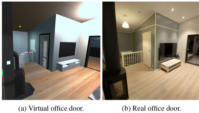
FIGURE 15. Real-time states of 2OfficeDoor, 2Stair, HueColorLamp2 located in the second floor, observed 21.02.2022. Note that the color of the spheres follows the same standards set in Fig. 4 and their positions represent the 3D position of the sensor in the physical asset.
