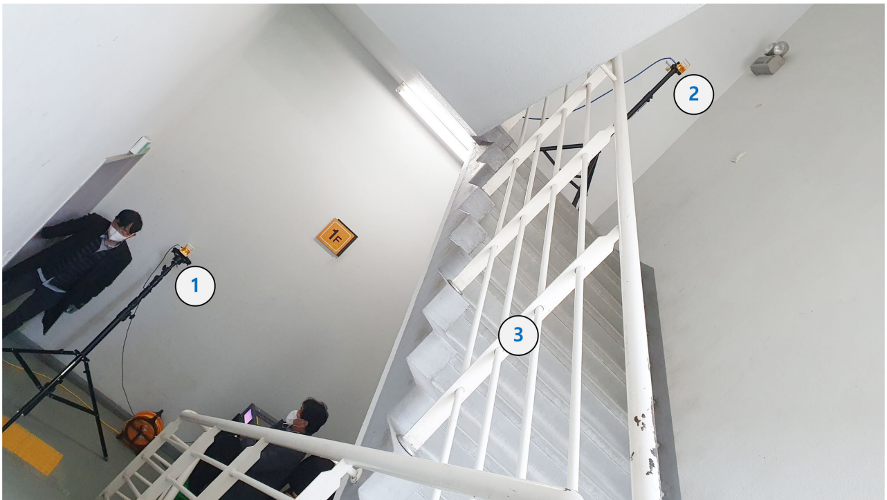
FIGURE 2. A measurement snapshot. In this scenario, the transmitting antenna is placed on the first floor, and the receiving antenna is placed on the second floor. Note: the position of the numbers ①, ②, and ③ respectively, indicates the transmitter, receiver and the metal protection frame of the stair.
