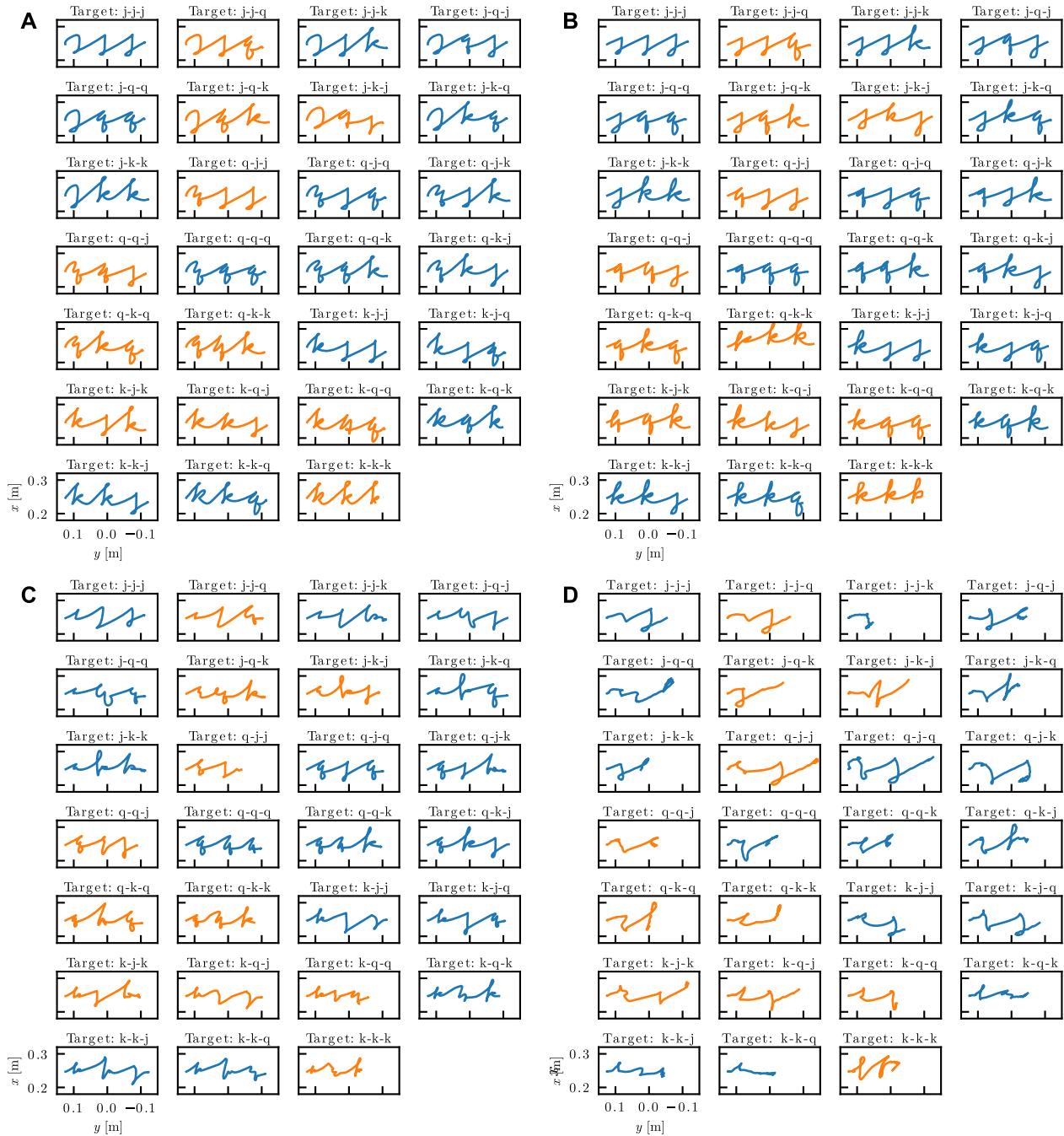
FIGURE 11. Generated trajectories by the robot. The trajectories in orange were not used in training. Proposed model with A: N = 4, K = 25 , B: N = 6, K = 10 , and C: N = 3, K = 80 ; D: baseline-B model.
