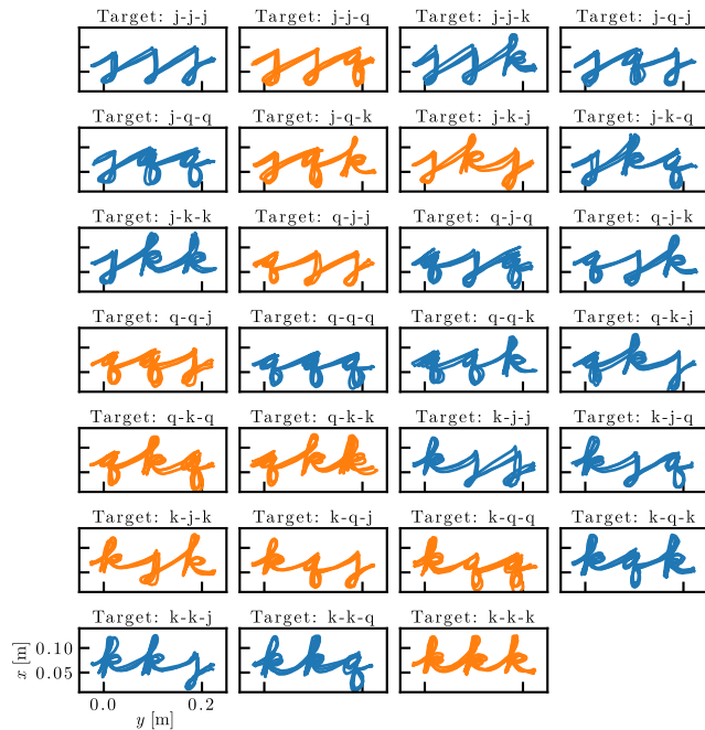
FIGURE 4. Collected demonstrations. Three demonstrations are collected for each pattern (overlaid). The orange patterns are excluded from synergy extraction or training.
