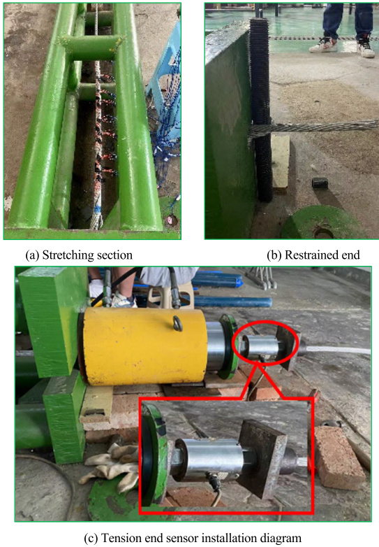
FIGURE 18. Tensile testing machine used in the experiment (from the company project test diagram).
