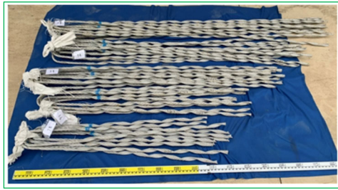
FIGURE 17. Preformed helical fitting sample used in the experiment.
