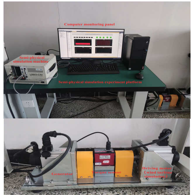
FIGURE 20. Experimental platform of PMSG semi-physical simulation.
