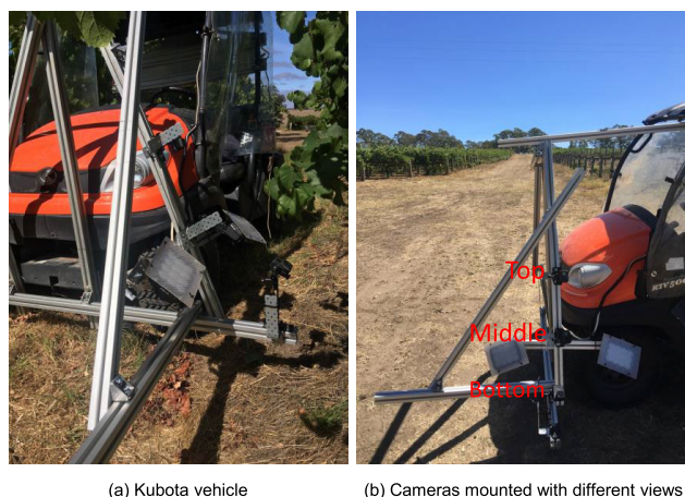
FIGURE 5. (a) Kubota vehicle used for video data collection. (b) Three different cameras are mounted on the vehicle.
