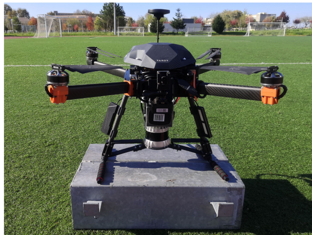
FIGURE 17. CROW UAV and its sensors payload: a monocular camera and a 3D LiDAR.
