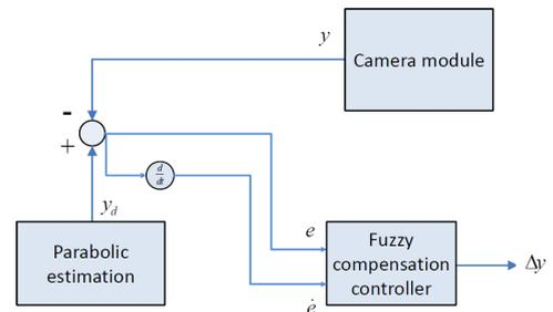
FIGURE 2. Tracking system architecture diagram.
