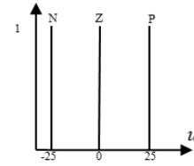
FIGURE 4. Output membership functions of the fuzzy compensator.
