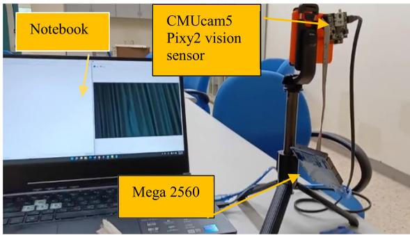
FIGURE 8. Full view of the experimental hardware system.
