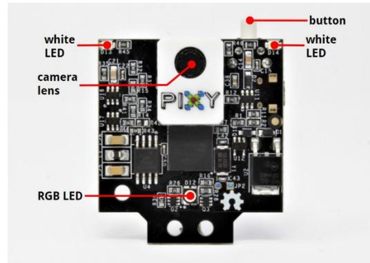
FIGURE 5. CMUcam5 Pixy2 vision sensor [21].
