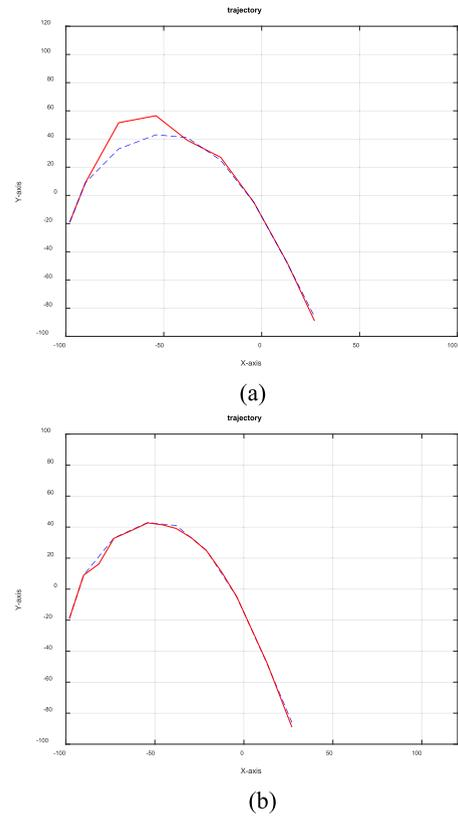
**FIGURE 15.** Third test dataset: (a) Experimental results without the fuzzy compensator. (b) Experimental results with the fuzzy compensator.
