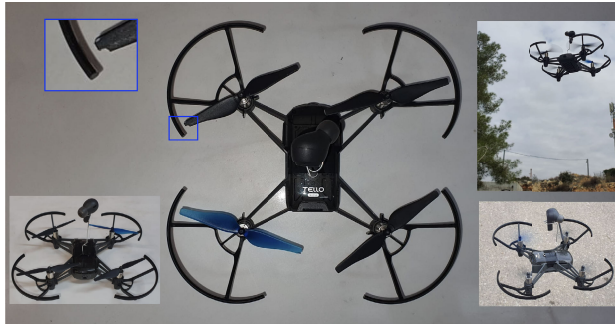
FIGURE 1. A standard BLE (Bluetooth Low Energy) earphone is used as a “stethoscope” for sensing the drone’s “well-being”. The middle (main) image shows a Tello micro drone (sub 100 grams) with an earphone located a few centimeters above it (see also the lower left image). A minor anomaly in the propeller “tip” is shown in the upper left image. Another (more visible) anomaly is demonstrated by the blue propeller (which has slightly different parameters than the black ones). On the right side - two examples of the experiments are presented in outdoor scenarios; the upper image shows a relatively high altitude flight (about 8 meters above the ground, to avoid “ground effects”) and the lower left image shows the drone flying in a low altitude (about 1 meter above the ground).
