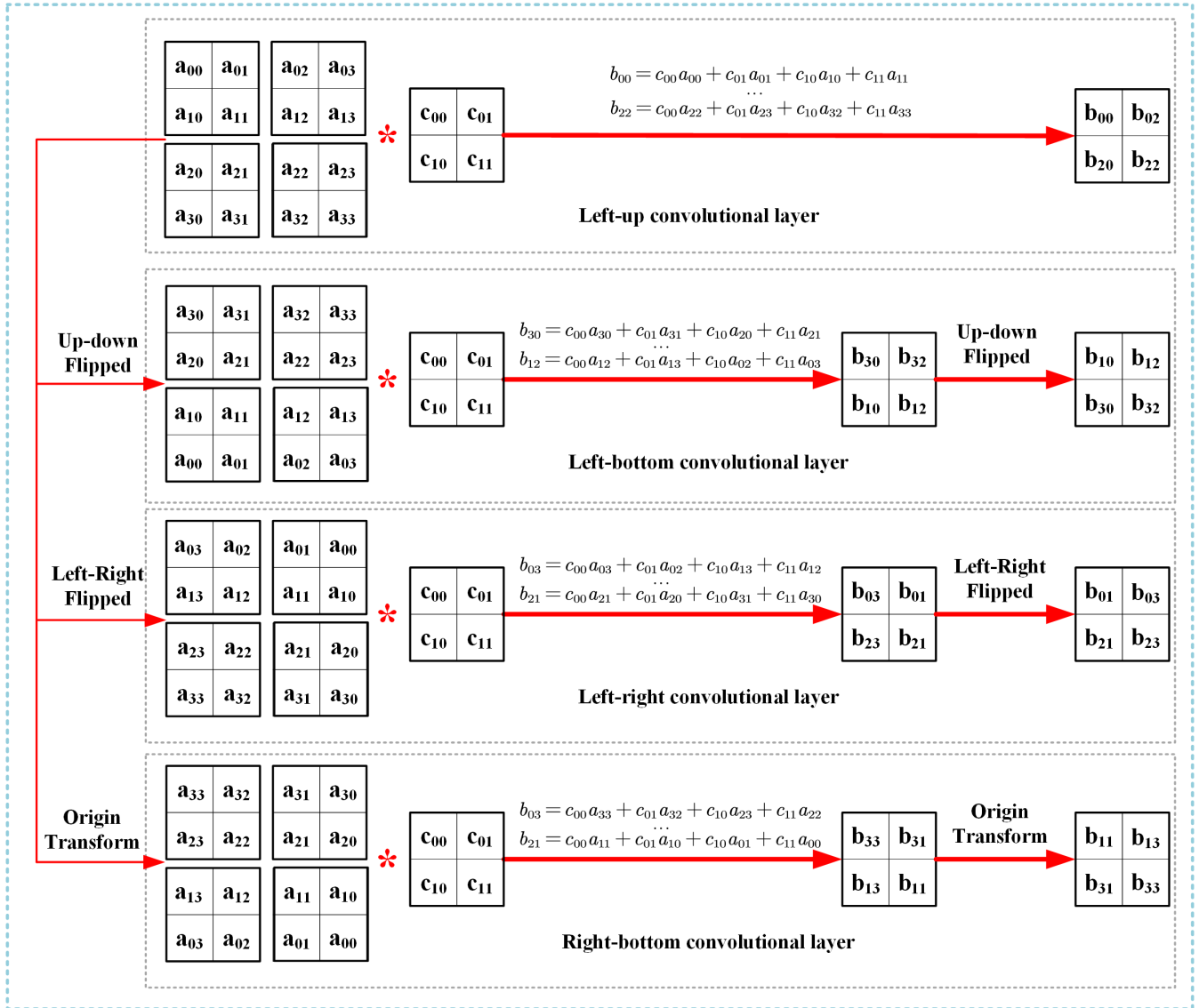
FIGURE 3. The proposed VS-LFAFE is implemented using four 2 \times 2 stride convolutional layers.
