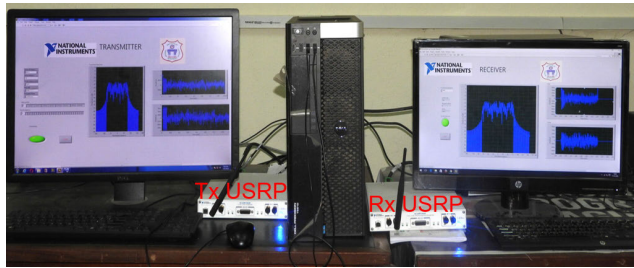
FIGURE 1. Set up used for demonstrating real-time transmission of GFDM system.
