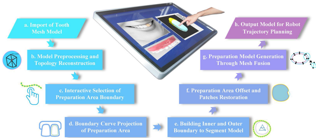
FIGURE 3. Digital interactive design scheme for preparations.
