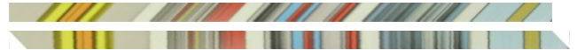
FIGURE 2. Top: EPI for (v_0, t_0) = (256, 0) with dimensions 17 \times 1024 ( s \times u ) for the Tarot light field with dimensions 17 \times 17 \times 1024 \times 1024 ( t \times s \times v \times u ). Bottom: EPI slanted so that EPI lines are almost vertical.
