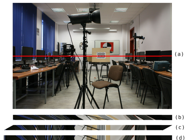
FIGURE 5. (a) Laboratory1 light field top left view, (b) s \times u EPI at line 644 (highlighted in red), (c) slanted EPI, and (d) slanted and padded EPI - with stretched s dimension for better visualization.
