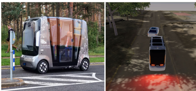
FIGURE 8. Vehicle digital twin representation. The real vehicle is on the left side, while its digital twin is on the right.
