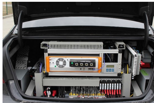
FIGURE 5. Data logging setup in a vehicle trunk.
