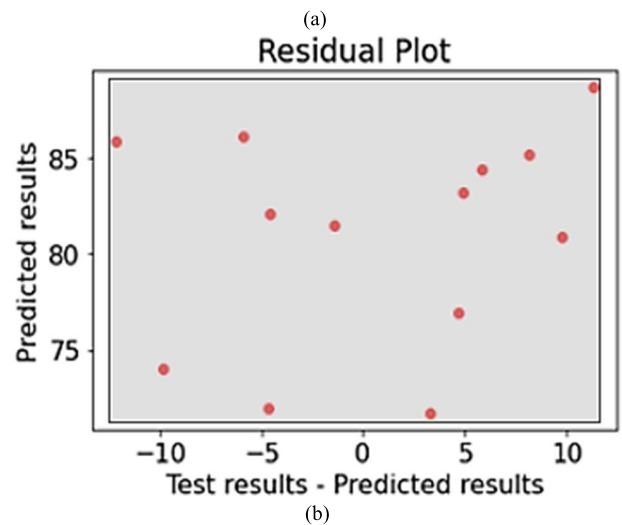
FIGURE 10. (a) Calculated and predicted ablation percentage using simple regression (b) Residuals plot with maximum error in ablation percentage prediction of 13 percent.
