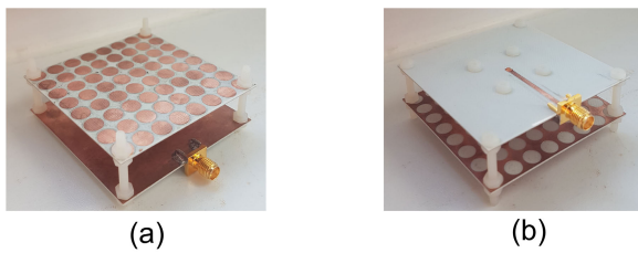
FIGURE 16. Fabricated Wideband polarization independent RCA (a) Top view (b) Bottom view.
