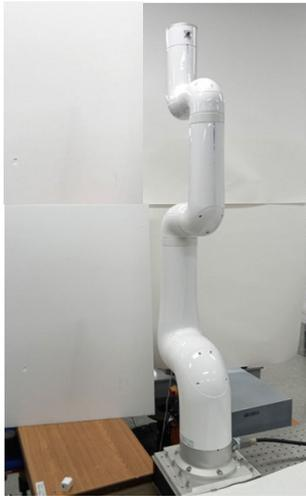
FIGURE 11. Indy7 6-DOF robot experimental platform.
