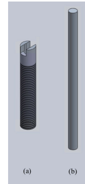
FIGURE 2. Modified Tuning Pins (MTPs): (a) Hollow M4 tuner used for a manual tuning of cavities and coupling windows; (b) Inner pin used to short circuit cavities or coupling windows by inserting it in the hollow M4 tuner.
