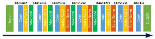
FIGURE 9. A discriminator structure designed with PatchGAN as the basic structure. Conv means convolutional layer, Maxpool means maximum pooling layer, BatchNorm means BN layer.
