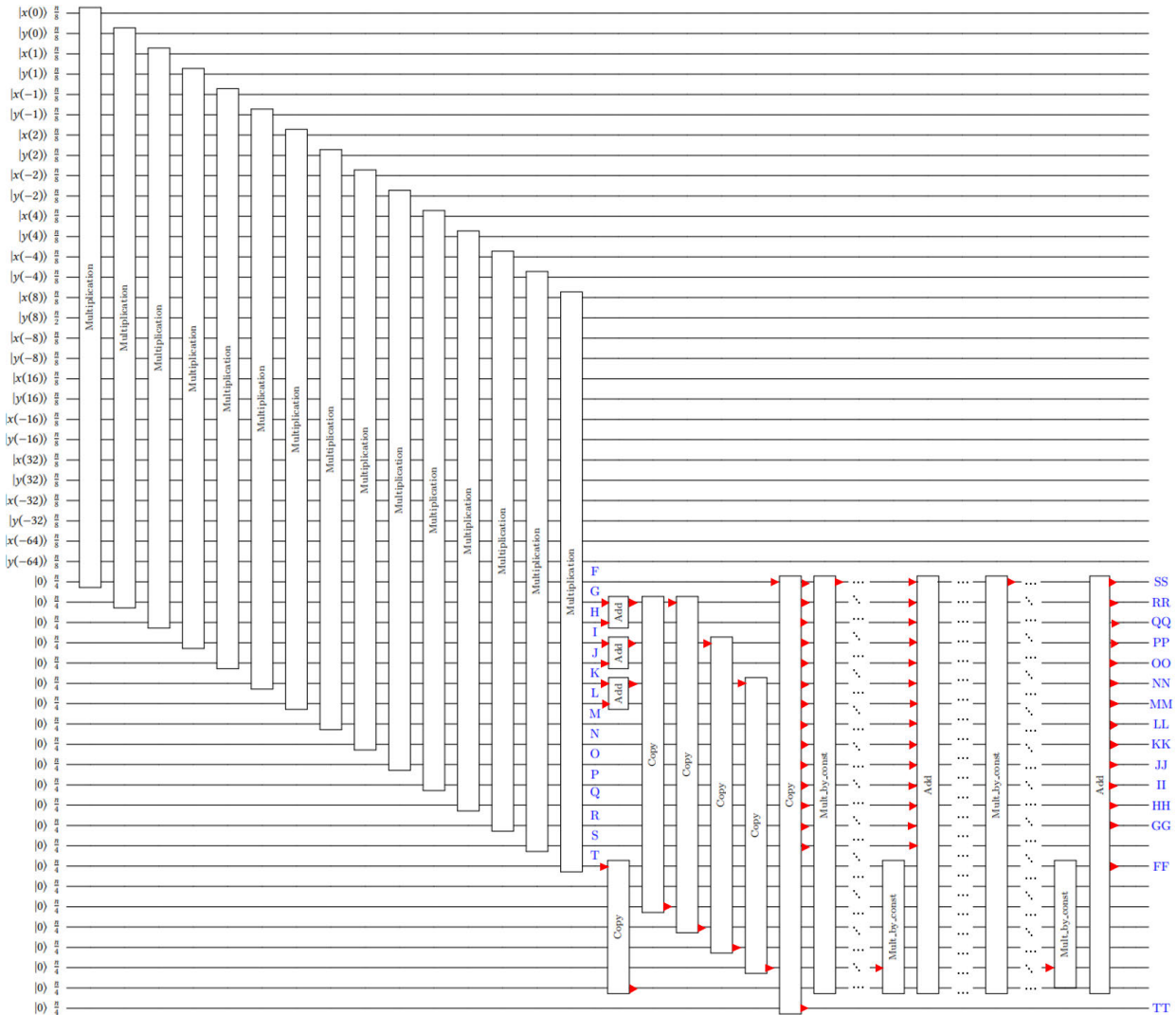
FIGURE 8. Quantum circuit consisting of point-wise multiplication and the interpolation of the Toom-Cook 8-way. The image depicts, in the form of function block boxes, the six different processes that, when combined, make up the Toom-Cook 8-way quantum circuit. The operations consist of copying, subtracting, adding, shifting, and sub-multiplying the data.
