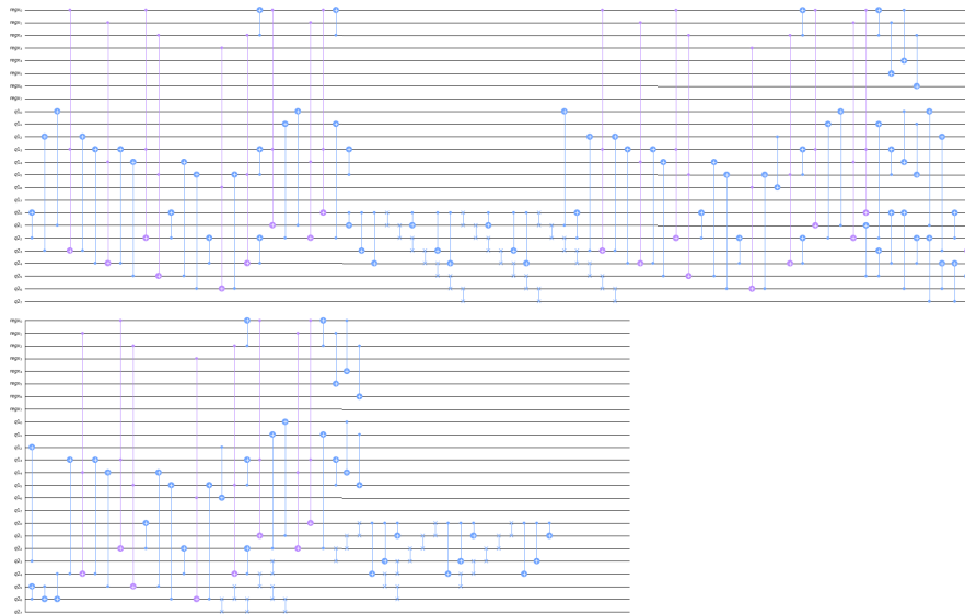
FIGURE 1. Karatsuba’s improvement multiplication with the highest degree polynomial is m = 8 . On a 64-bit Windows 10 Pro (Intel i7-8700, six-core CPU) with 64 GB of RAM and Python 3.9.7, the quantum circuit yields from the Qiskit simulation.
