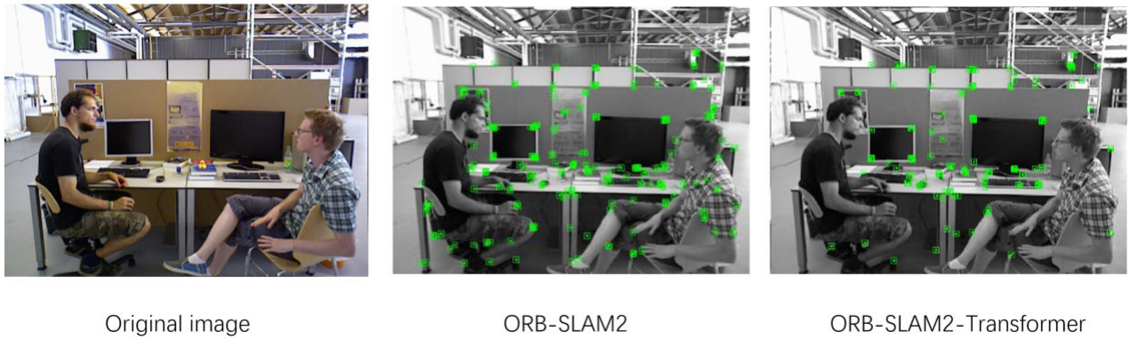
FIGURE 5. Typical examples for the results of dynamic points projection on TUM data set.
