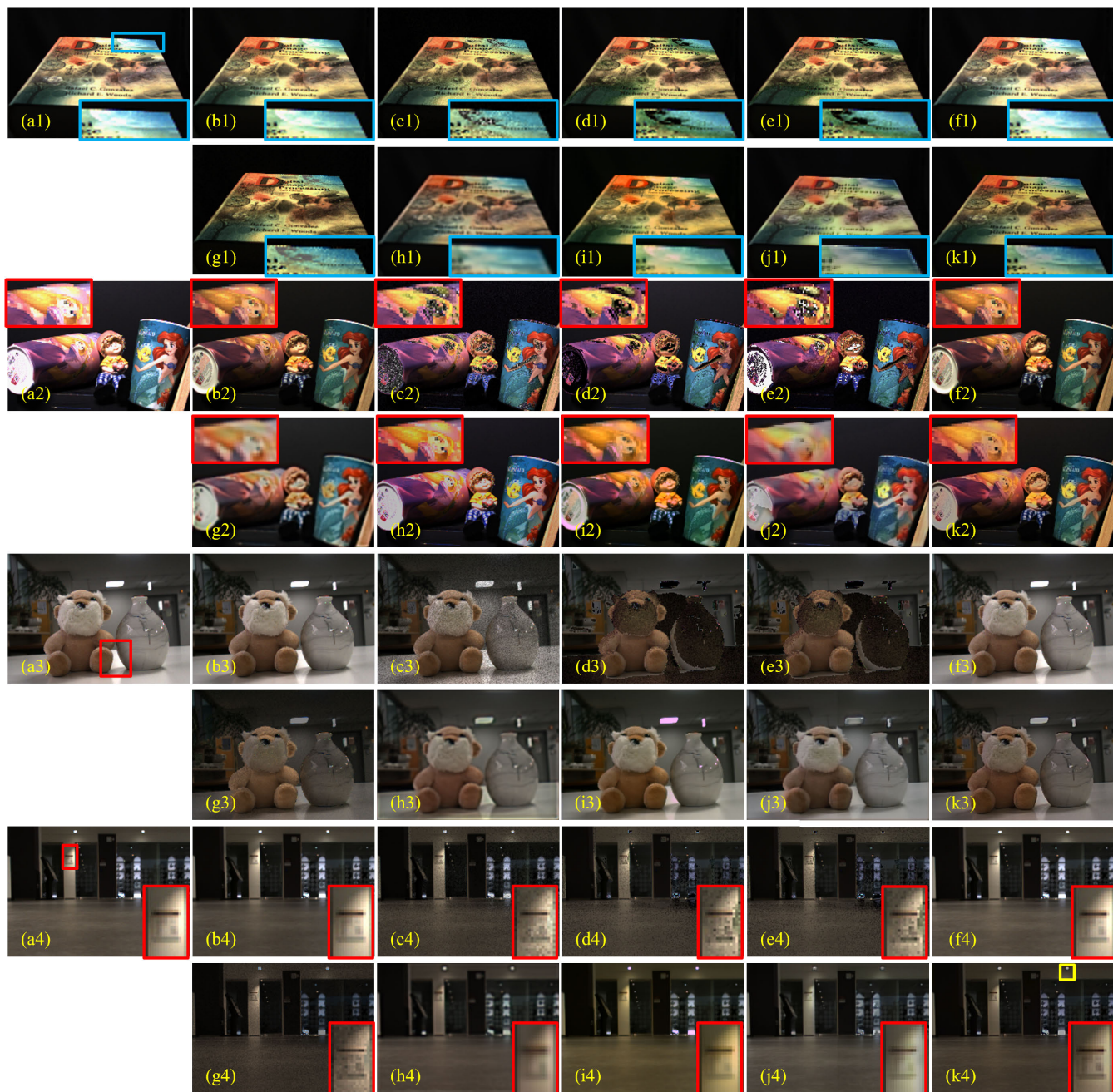
FIGURE 7. (a1-a4) input image, (b1-b4) TDP, (c-j) the diffuse reflection of (c) Akashi and Okatani [41], (d) Yamamoto and Nakazawa [42], (e) Yang et al. [43], (f) Tsuji [33], (g) Fu et al. [44], (h) JSHDR [39], (i) Yoo et al. [17], (j) JSHDR-Trans [45], (k) the proposed method.
