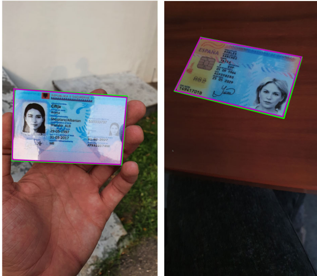
FIGURE 6. Images from MIDV-2020 dataset with document quadrangles: green for ground truth, and magenta for the detected in our experiments.
