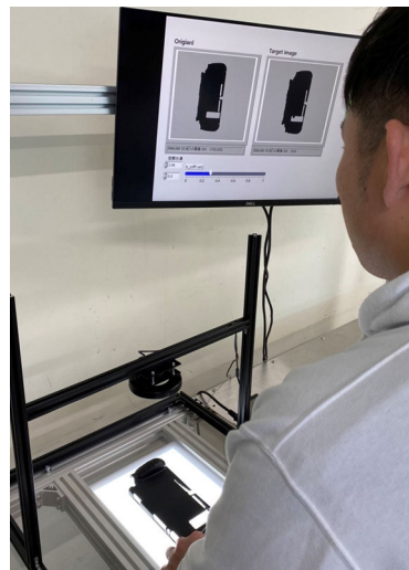
FIGURE 1. Overview of the visual inspection of a rough-alignment plastic part.
