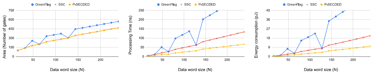
FIGURE 10. (a) Area (in number of 1x Inverter gates), (b) Computation latency in nanoseconds and, (c) Total energy consumption (Static + Dynamic) in nanojoules. Results compiled by leveraging post-synthesis reports in 45nm technology.
