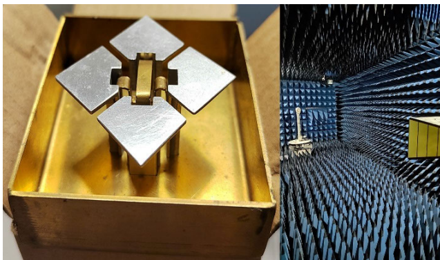
FIGURE 9. Photographs of the fabricated antenna and measurement in the anechoic chamber.
