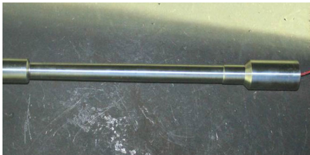
FIGURE 6. Engineering prototype of penetrating system before coating the outer layer with carbon fiber.
