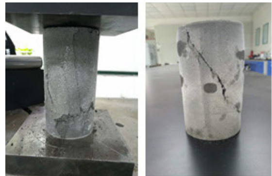
FIGURE 7. UCS test of simulated lunar water ice with different moisture content and at different temperature.
