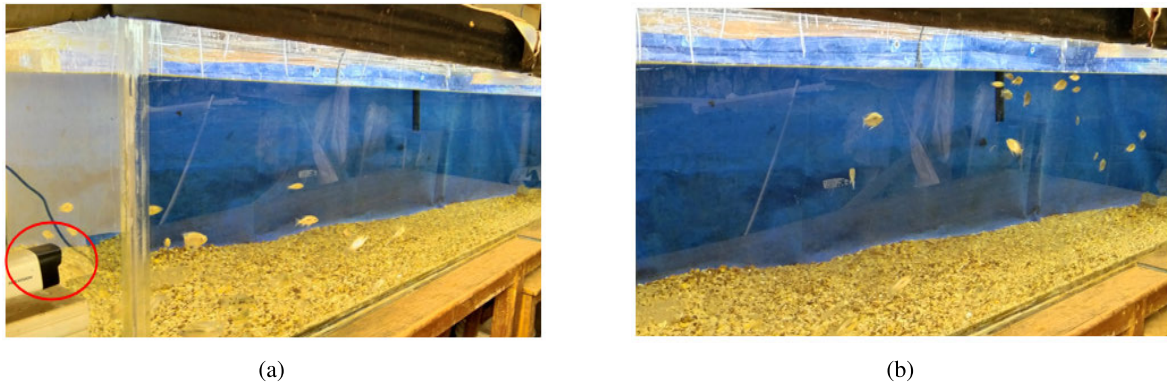
FIGURE 2. Experimental setup for collecting the dataset. (a) Sample image of aquarium with camera highlighted in the red circle. (b) Sample image of aquarium with blue HDPE sheets and sand bed.
