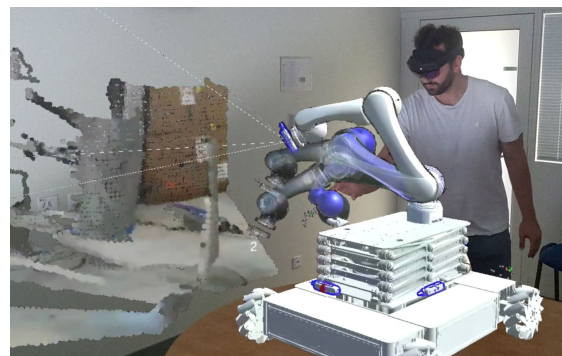
FIGURE 7. Local collaboration scenario with two operators in the same room. The figure shows the viewpoint of one operator on the scene and the second operator that controls the robot. In this example, the controlling operator created a trajectory with waypoints to approach a target in the real environment.
