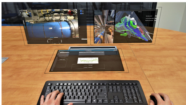
FIGURE 11. A virtual control centre projected in the AR workspace. The 2D and 3D interface type, computer screen visualisation, keyboard, and mouse are used.
