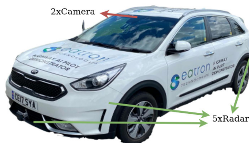
FIGURE 2. Target vehicle platform with multiple cameras and radar sensors.
