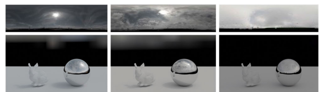
FIGURE 1. HDR maps (top) reconstructed using the proposed method under three weather conditions (left: clear, mid: cloudy, right: overcast); the images rendered using the reconstructed HDR maps (bottom).
