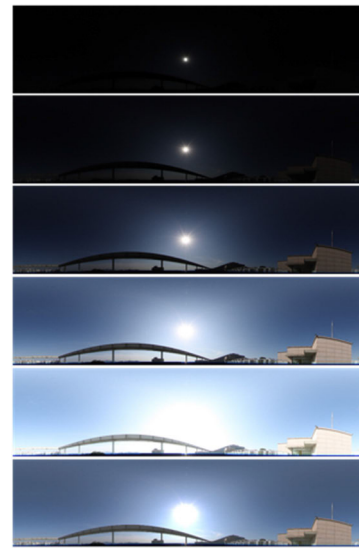
FIGURE 10. Images of a given scene captured with five exposure values, and the corresponding synthesized HDR map (the last row).
