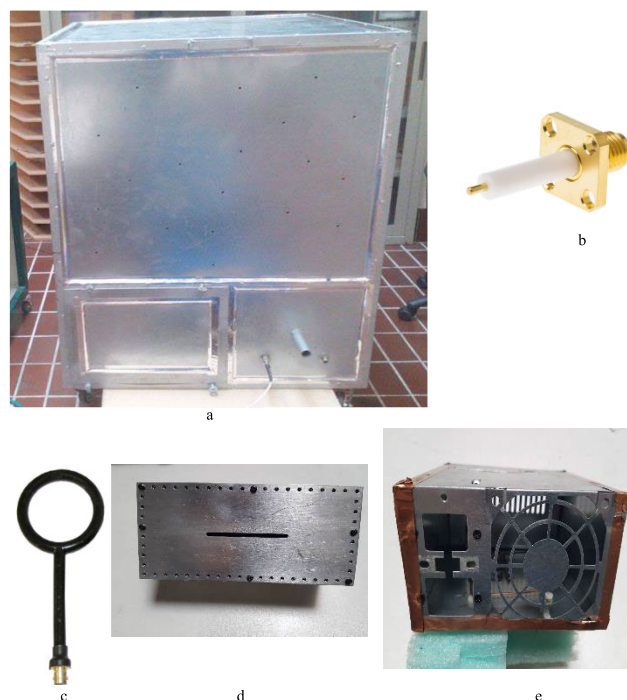
FIGURE 2. The reverberation chamber (a), the monopole antenna (b), the loop (c), the metallic box with a slot (d) and the chassis of a power supply (e).
