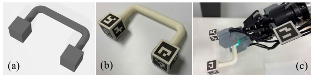
FIGURE 8. (a) CAD model of the 3D printed object. (b) Markers are attached to the end cubes. (c) Experiments in action.
