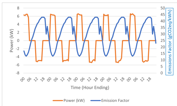
FIGURE 12. Power vs emissions in V2B arbitrage test.
