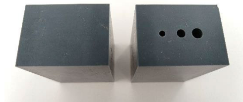
FIGURE 9. Photography of Sample 1(a) and 1(b) made from Polyvinylchlorid (PVC): 30 mm \times 40 mm \times 60 mm (b) hole diameters: 3, 4, and 5 mm.
