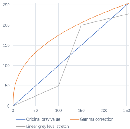
FIGURE 5. Gray value curve of linear grey level stretch and Gamma correction.
