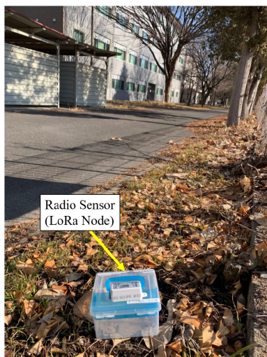
FIGURE 14. Radio sensor in 920 MHz band LoRa node.
