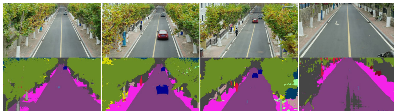
FIGURE 10. The actual scene segmentation from the drone’s low-altitude perspective (Based on QNet-attention+FlowNet2-s).
